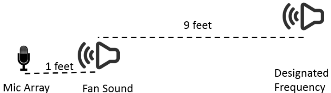
Figure 42: Diagram of sound channel prototype layout
