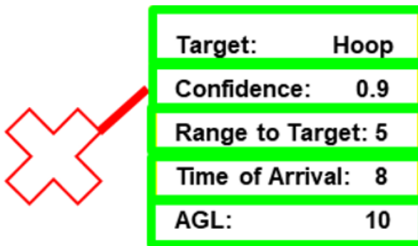
Figure 2: Symbology Example Metadata box and Red X for Target Identification, image referenced from Lockheed Martin DOMINANCE Kick-Off slides
